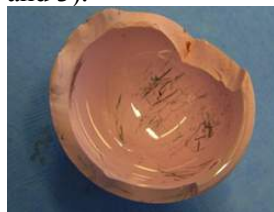
Fig. 2. This photograph shows a fractured BIOLOX®delta ceramic acetabular component with intense black synovial reaction.
