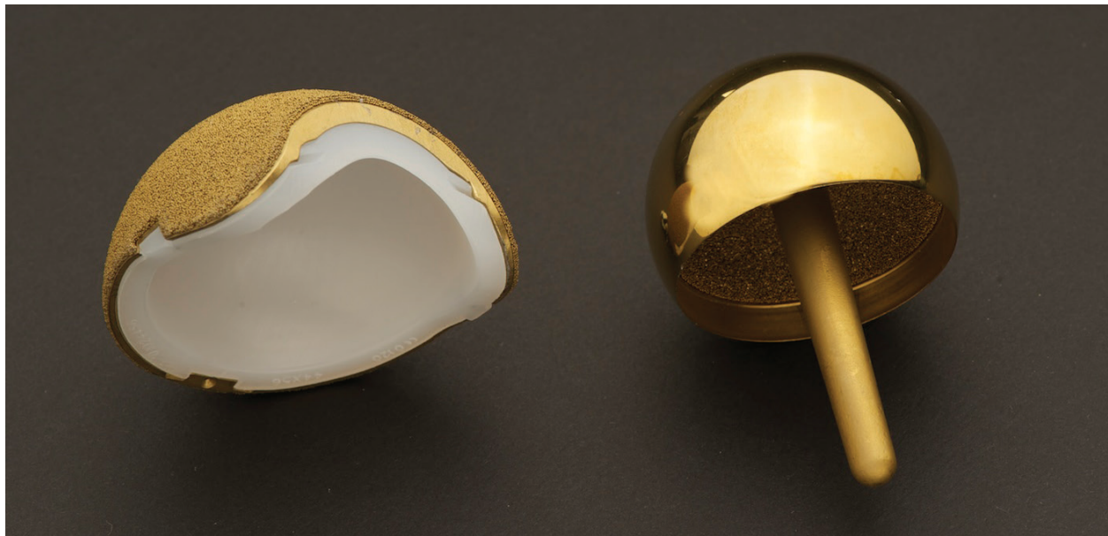
FIG. 1: Photograph of the two-piece TiN-coated acetabular component and femoral resurfacing that was tested to 30 million cycles.
