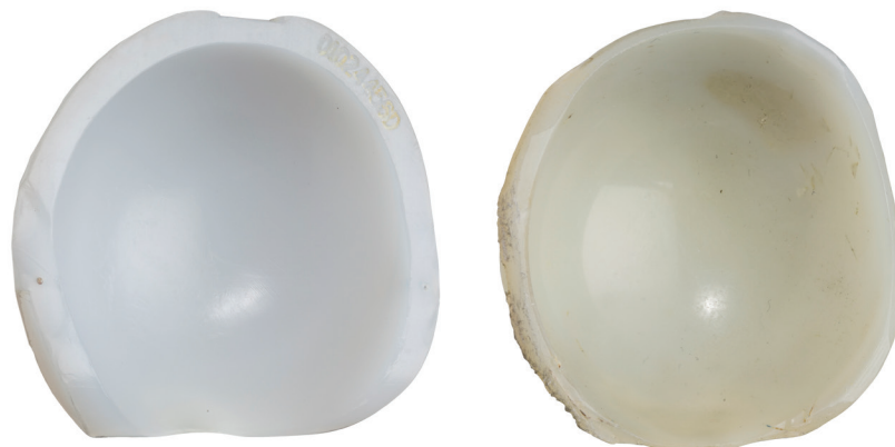
FIG. 2: Photograph showing XLPE (left) and ConvPE (right) inserts after 30 million cycles with PMMA challenge. Severe wear of the ConvPE can be seen.
