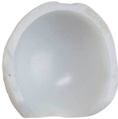
FIG. 3: Photograph of a tested acetabular component showing scratches on the XLPE after 30 million cycles. The original machine markings remain visible.
